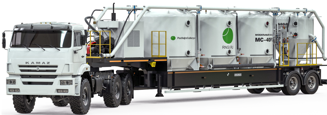
Figure 1 - MS-40R3-05 Mobile cement bulk storage.
