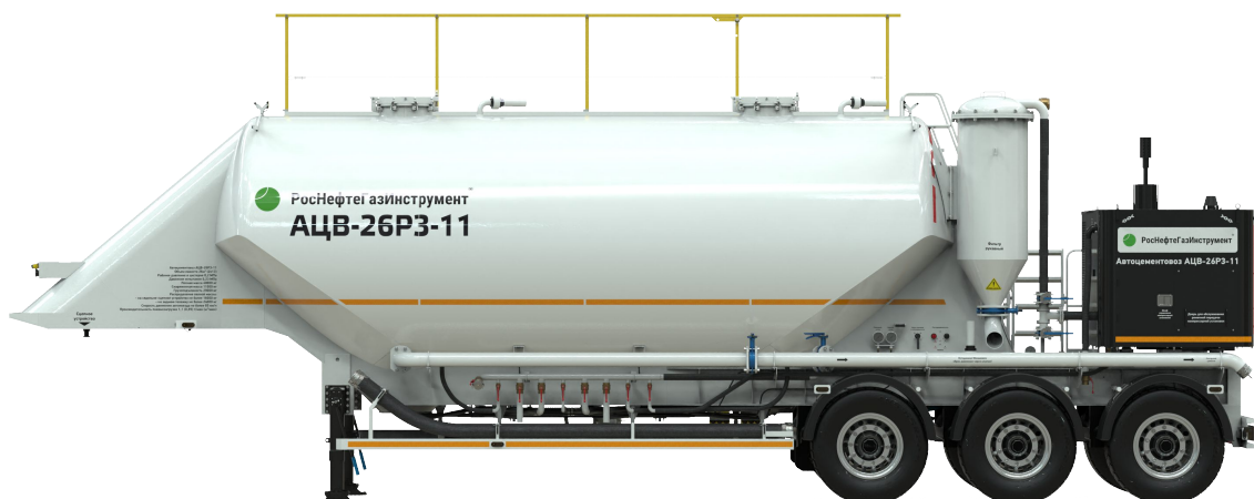
Figure 2 - ACV-26R3-11 bulk cement trailer.
